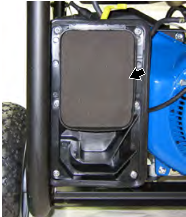
Figure 32 – Removing Fine Inside Air Filter
