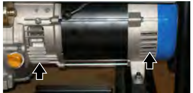
Figure 45 – Alternator Cooling Air Inlet and Outlet Port
