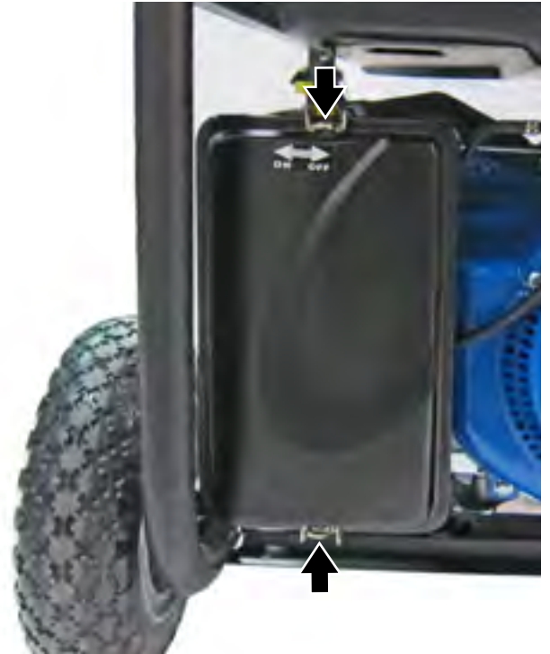
Figure 35 – Installation of Air Filter Cover
