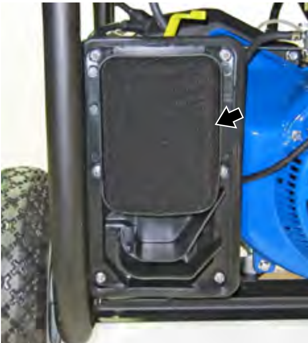
Figure 31 – Removing Coarse Outside Air Filter
