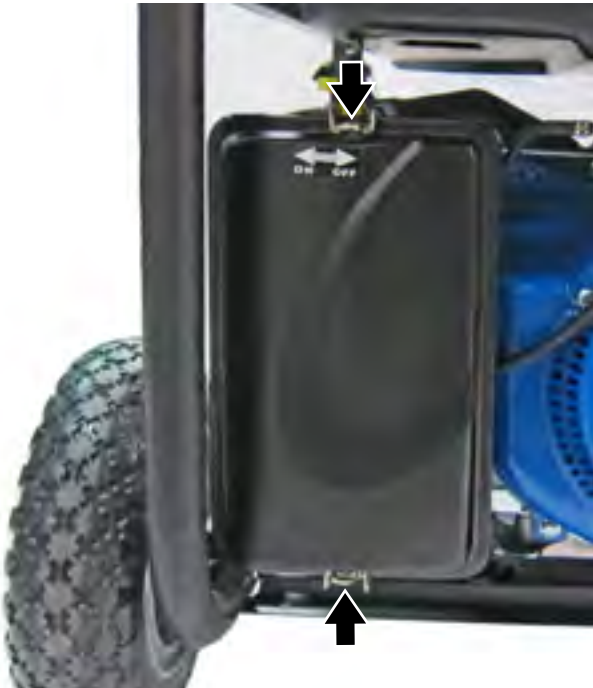
Figure 30 – Removing Air Filter Cover
